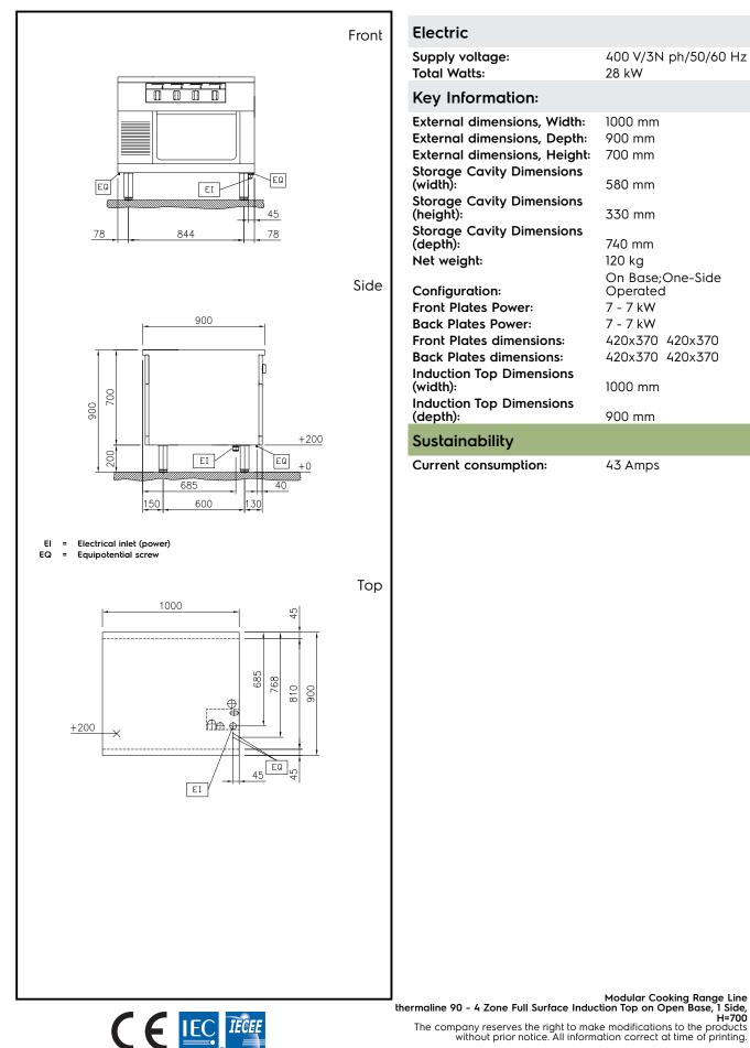
Modular Cooking Range Line thermaline 90 - 4 Zone Full Surface Induction Top on Open Base, 1 Side, H=700 The company reserves the right to make modifications to the products without prior notice. All information correct at time of printing.
